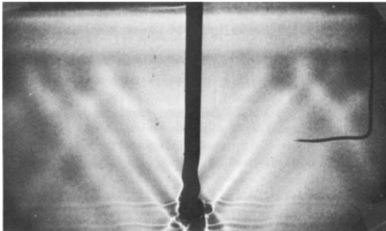
FIGURE 9. Experimentally observed ray patterns generated by an oscillating cylinder in an unsheared fluid. The density distribution for these runs is shown in figure 7. (a) \omega/N_0 = 0.40 ; (b) \omega/N_0 = 0.52 ; (c) \omega/N_0 = 0.82 .
