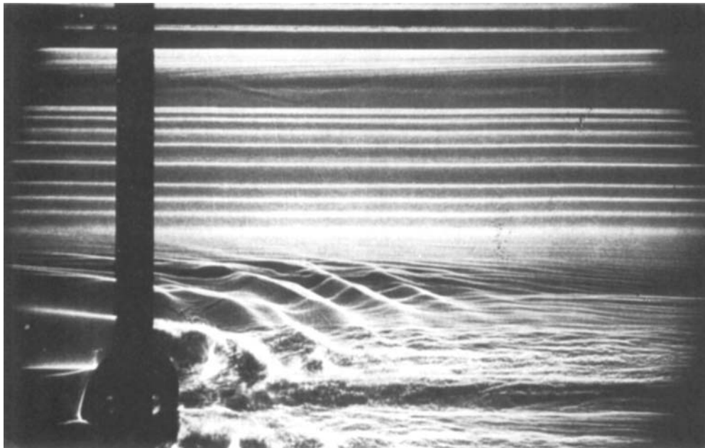
FIGURE 17. Enlargement of figure 16(c) showing detail of wave motion in the neighbourhood of the critical layer.
